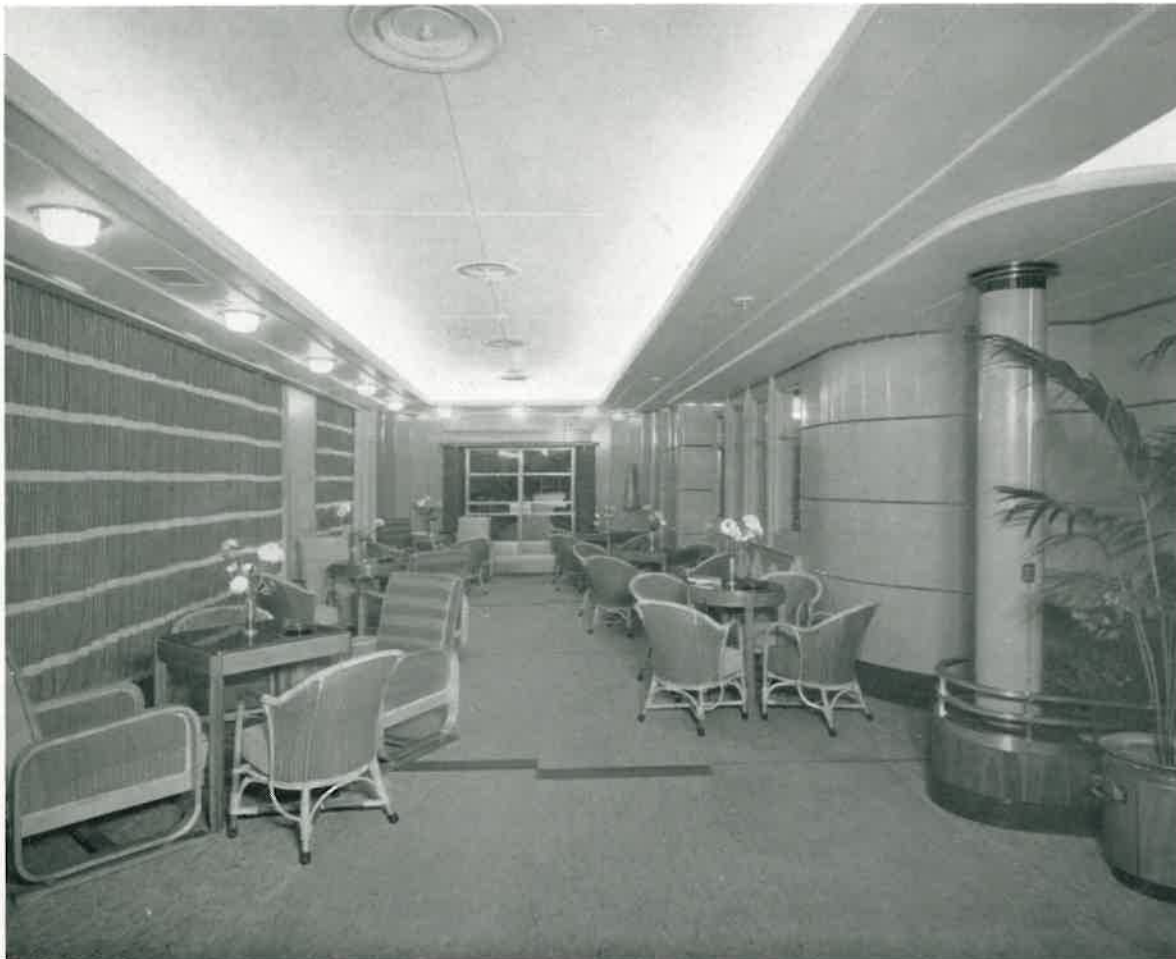
Fluorescent cornice lighting, combined with tungsten deckhead fittings, gives a soft illumination in the observation lounge where passengers can rest without the distraction of glaring lights above them.
