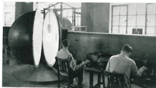
PHOTOMETRY. The lamp to be measured is operated inside a spherical enclosure whose white diffusing surface collects and mixes light from all around the lamp. A sample of this integrated light enters the inspection “tunnel” (seen on the right) and illuminates one half of the field of view; the other half is lit by a lamp of known optical characteristics.
