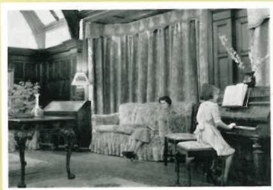
Indirect lighting from fluorescent lamps is used in this lounge of a centuries-old farmhouse.
